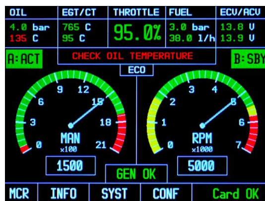
Figure 6-10: Warning “CHECK OIL TEMPERATURE” (Software 915iS RS11.00)
