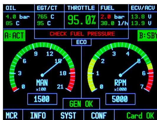
Figure 6-8: Warning "Check FUEL PRSSURE" (Software 915iS RS11.00)
