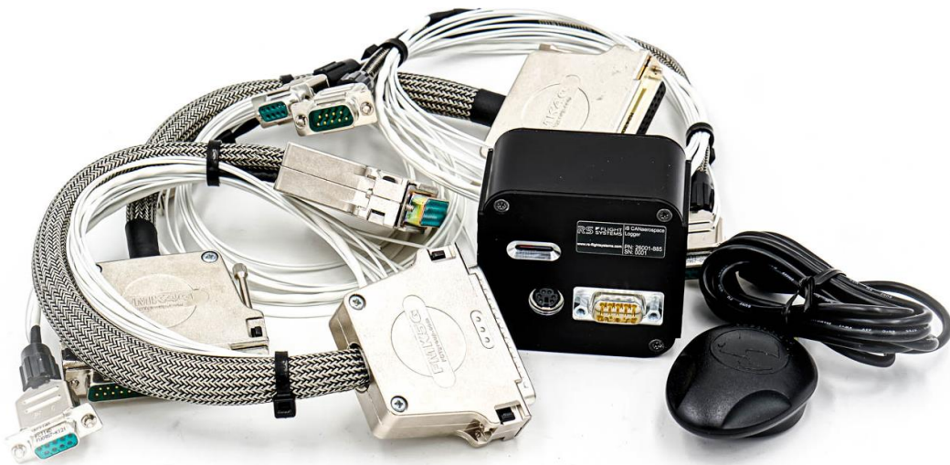
Figure 2-1: iS CANaerospace Logger with optional accessories
